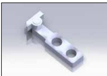
double bore hinged connector right with hinged head, for butt joints dim.: 12 x 48 x 3 mm steel, zinc-plated
