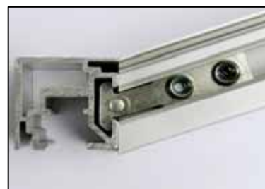
double bore hinged connector right with hinged head, for butt joints dim.: 12 x 48 x 3 mm steel, zinc-plated
