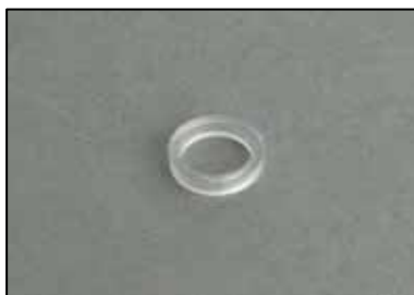
fixing aid, PA ring ext. Ø 9, int. Ø 6, width 2 mm Compressable 3-9 mm low-grip PA rings for securing threaded strips in place
