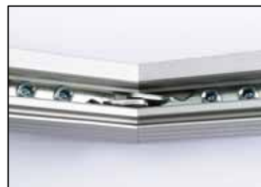
quadr. bore hinged connector vertical vertical, hinged connector for joining two sections at any angle dim.: 12 x 104 x 3 mm steel, zinc-plated
