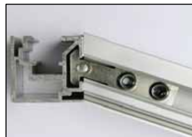
double bore hinged connector left with hinged head, for butt joints dim.: 12 x 48 x 3 mm steel, zinc-plated
