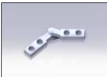
quadr. bore hinged connector flat, hinged connector for joining two sections at any angle dim.: 12 x 85 x 3 mm steel, zinc-plated
