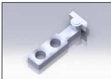
double bore hinged connector left with hinged head, for butt joints dim.: 12 x 48 x 3 mm steel, zinc-plated
